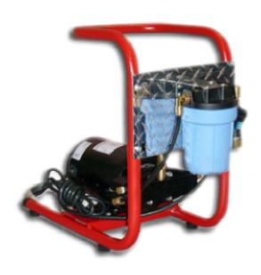
A compact direct drive pump assembly for commercial or residential installations. The low noise level makes it easy to work with. Features auto shut off solenoid, internal adjustable pressure regulator (200-1000 psi max.) Has a 8-136 nozzle capacity depending on model.
